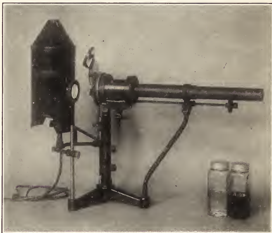
FIG. 53 Instrument for measuring clarity
