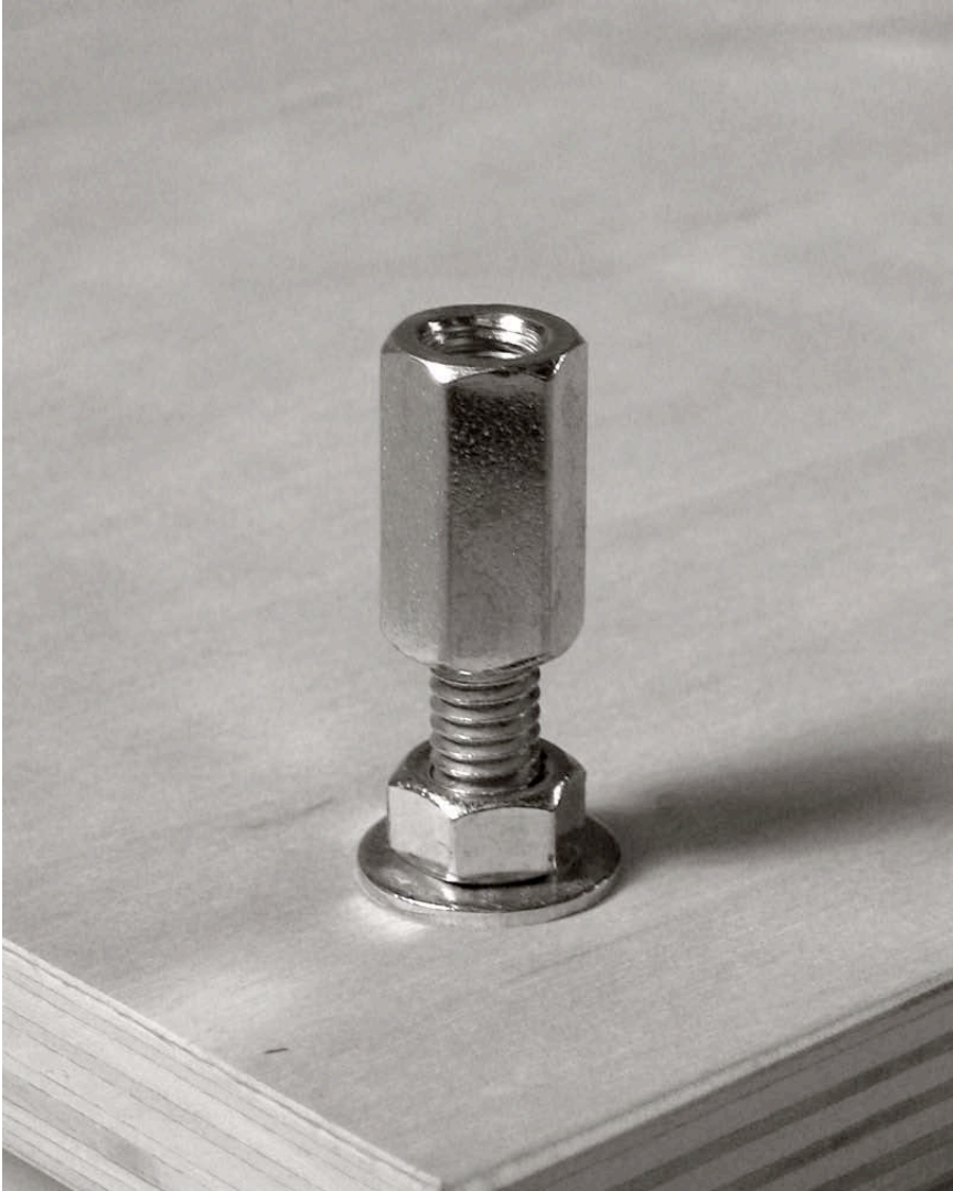
Detail of adjustable leveler. It is made by inserting a bolt into a countersunk hole from the other side of the plywood. The washer and nut secure the leveler to the wood plate and the hexagonal connection nut adjusts for height.
