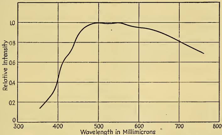
FIG. 3.—Relative spectral intensity of mean noon daylight at Washington, D. C.
