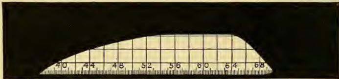
FIG. 6.—Color-sensitivity curve for emulsion B. (Eastman Kodak Co.)
