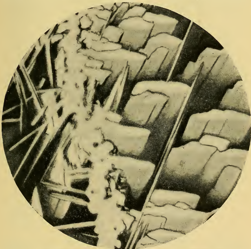
FIG. 16.—A three-dimensional picture of manganese steel, water toughened and drawn at 750°C. (Magnification, 3500 \times .)
