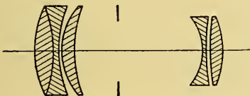
FIG. 56.—Taylor-Hobson 2.3\times , f/5 distortionless telephoto.
