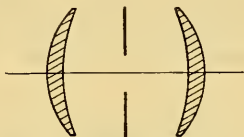
FIG. 4.—Steinheil's periscopic lens.
