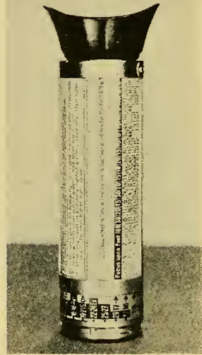
FIG. 6.—Bewi Sr. visual exposure meter with focusing eyepiece. This meter has a blue filter and viewing screen covering the average field of view, which enables the photographer to obtain a good idea of what his photograph will look like and at the same time enables him to determine exposure.
