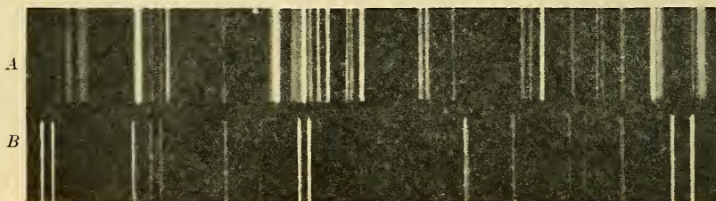
FIG. 14.—Spark A and arc B spectrograms made under identical conditions.
