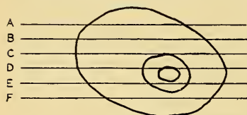
FIG. 22.—Diagram showing method of optical sectioning with the ultraviolet microscope.
