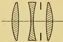
FIG. 27.—Cooke lens with negative element mounted between positive elements.
