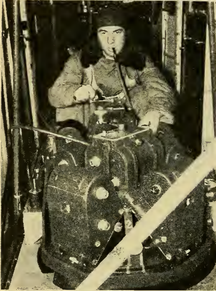
FIG. 6.—Nine-lens camera for making aerial photographs, mounted in floor of plane. Note oxygen arrangement.
